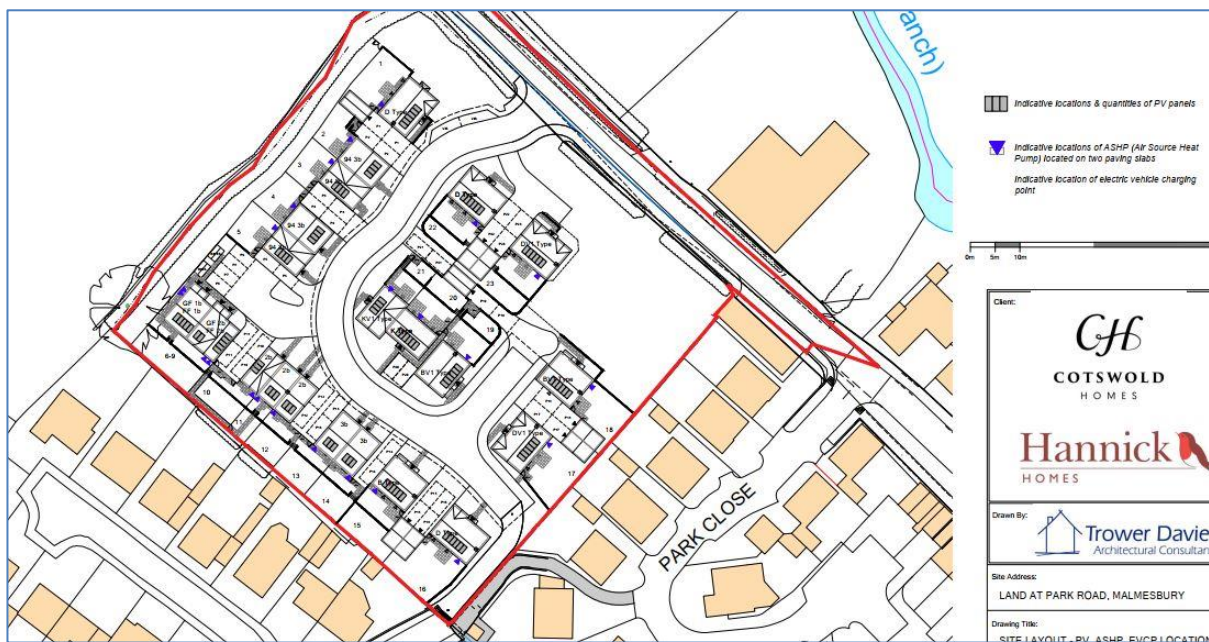
8 Indicative plan showing solar, ashp & car charging
