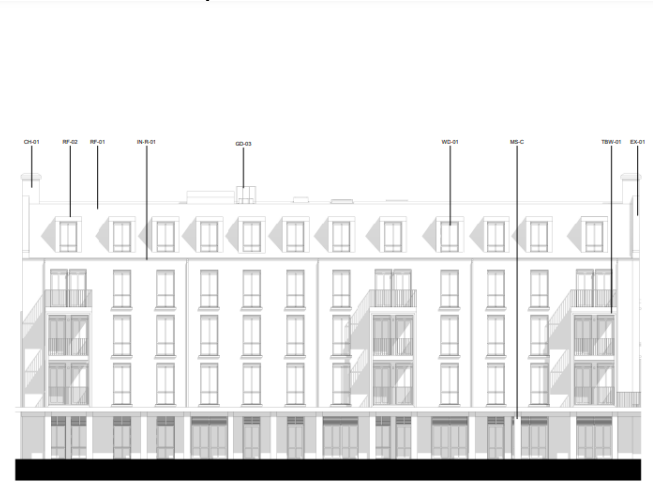
Building A - North Elevation 1:100
