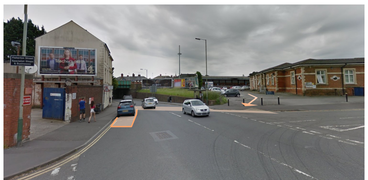
Image 4: Pedestrian and cycle access to/from station to bus stops shown. South Bound Bus Stop to be relocated and junction redesigned with crossing to allow easy crossing.
