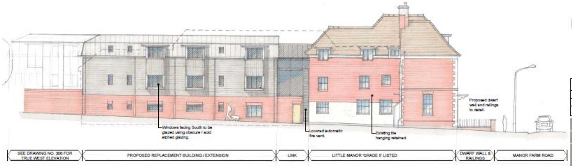
Proposed South Elevation Scale: 1:100 @A1 (1:200 @A3)
