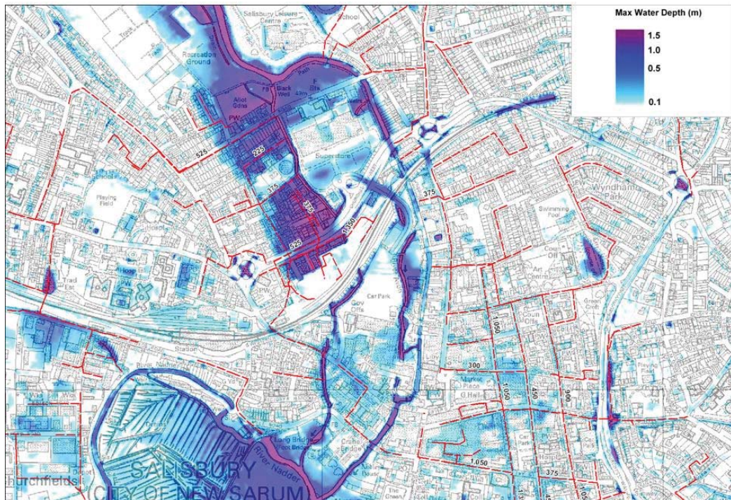
Figure 7-12: Wessex Water surface water sewer location and approximate diameters (in mm) within the vicinity of the Churchill Way. Pluvial modelling results for the 1% AEP rainfall event inclusive of climate change.
