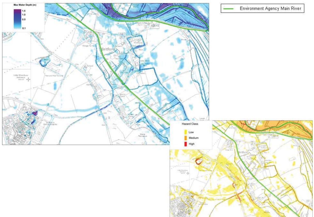
Figure 7-14: Pluvial modelling results during the 1% AEP event, inclusive of climate change (maximum depth and hazard) for the ordinary watercourses in Britford
