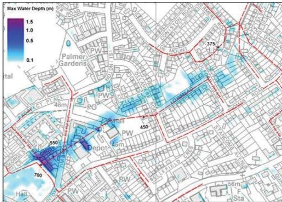
Figure 6-5: Wessex Water surface water drainage network in the vicinity of Timbrell Street. Surface water sewer shown as a red dashed line. Pluvial modelling results for the 1% AEP rainfall event inclusive of climate change.
