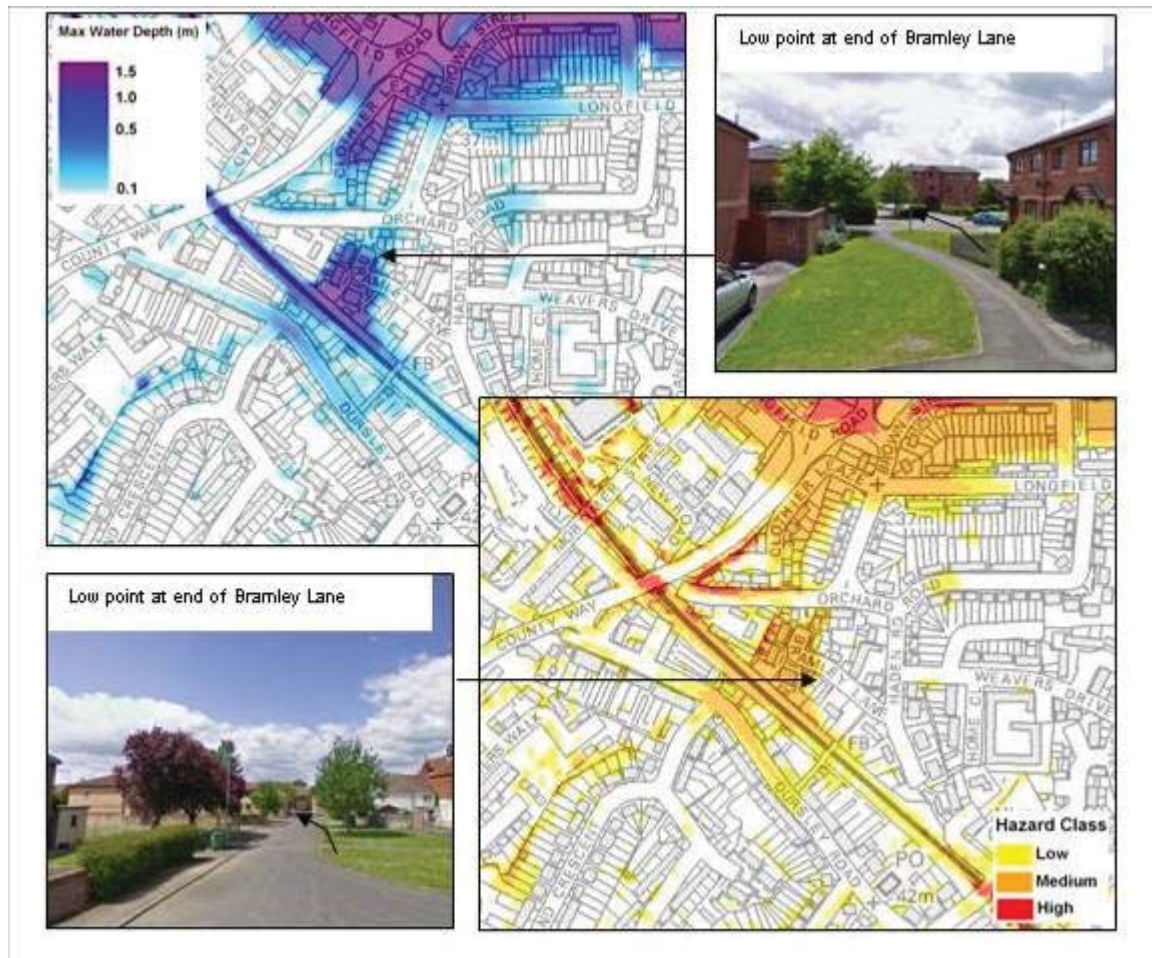
Figure 6-4: Pluvial modelling results (maximum potential depth and hazard) for the 1% AEP rainfall event including an allowance for climate change for the Bramley Lane Area.
