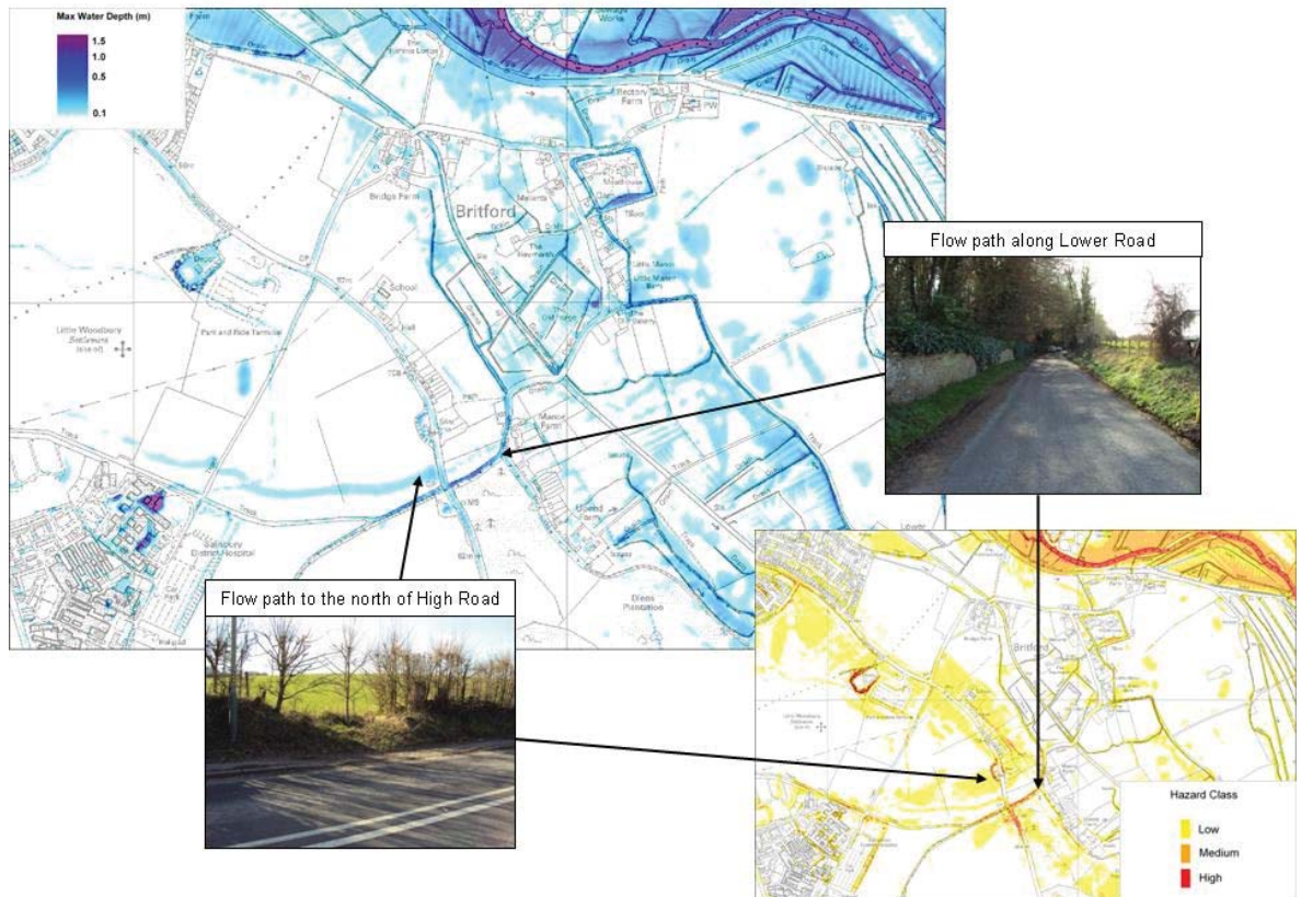
Figure 7-3: Pluvial modelling results (maximum depth and hazard) from the 1% AEP rainfall event inclusive of climate change for the Britford Area, southern Salisbury
