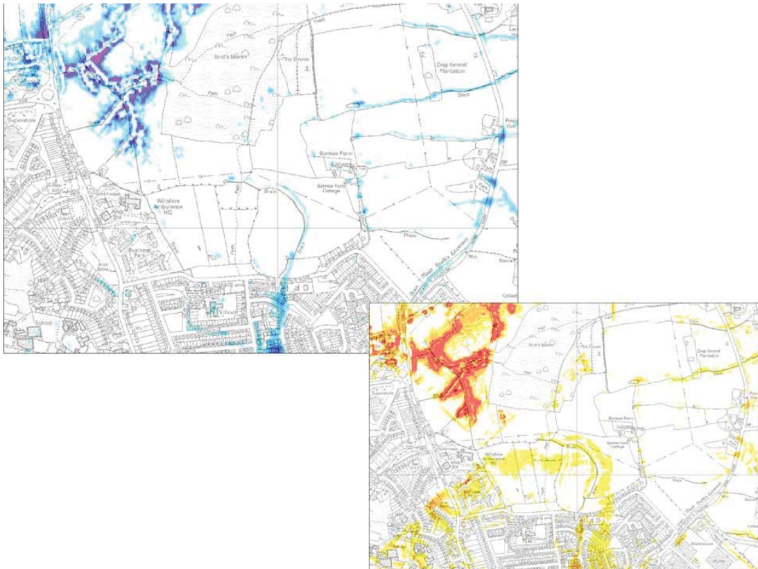
Figure 5-12: Pluvial modelling results during the 1% AEP rainfall event, inclusive of climate change (maximum depth and hazard) for the Hill Corner Road Farm Area
