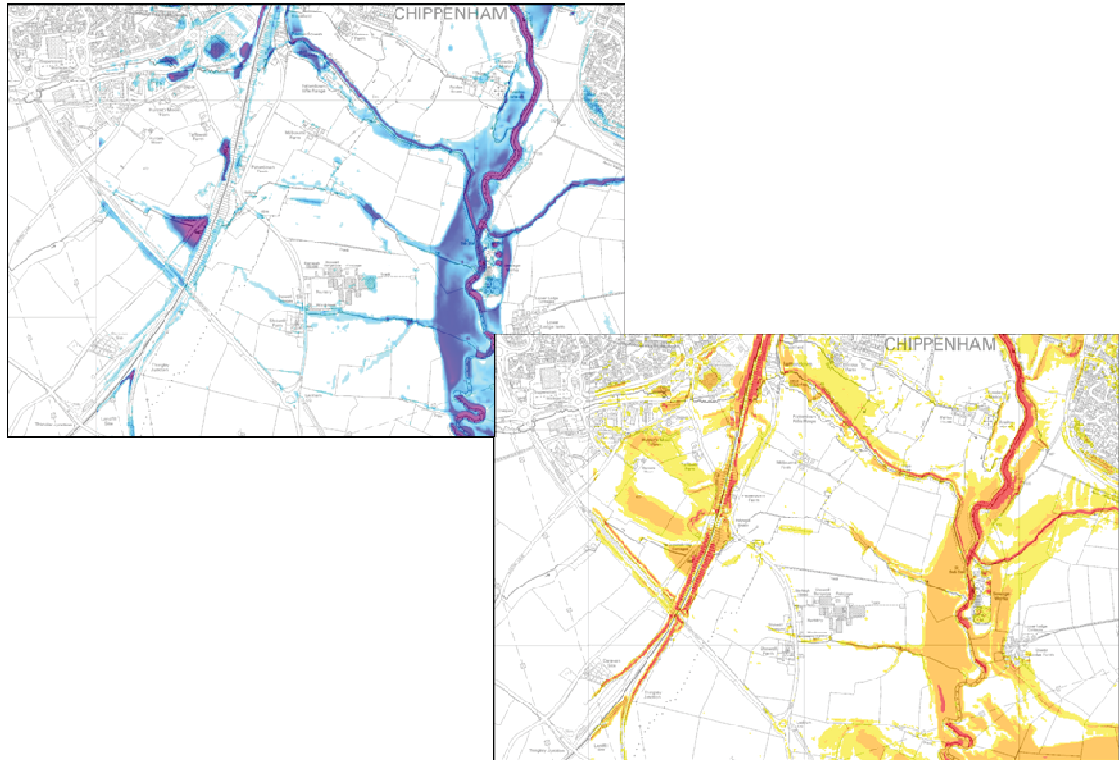
Figure 5-11: Pluvial modelling results during the 1% AEP rainfall event, inclusive of climate change (maximum depth and hazard) for the Patterdown Area
