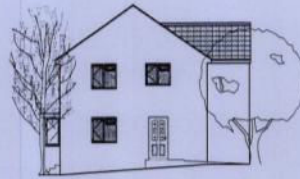
PROPOSED SIDE ELEVATION
