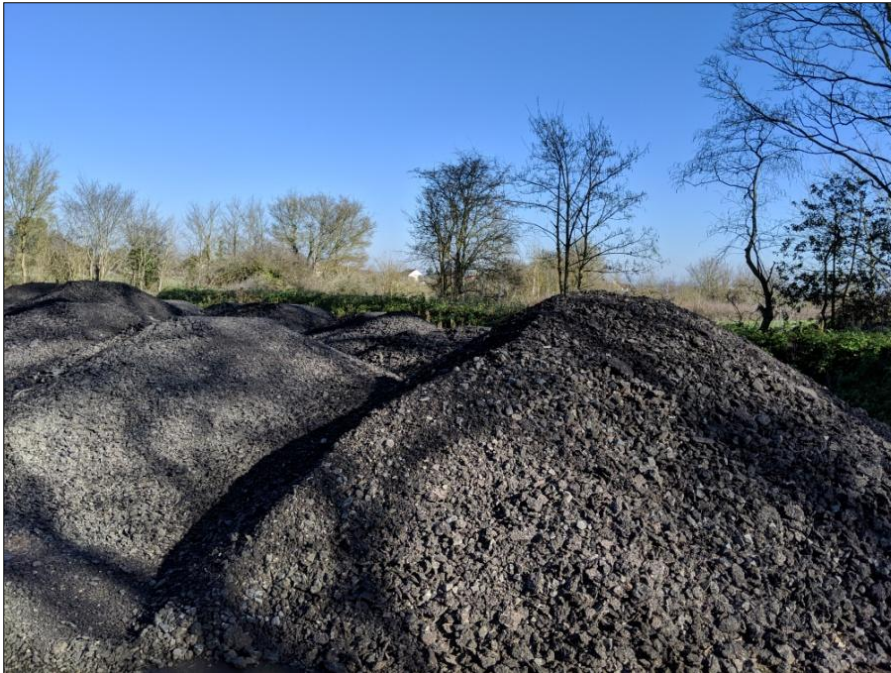
Road planings ready for reuse
