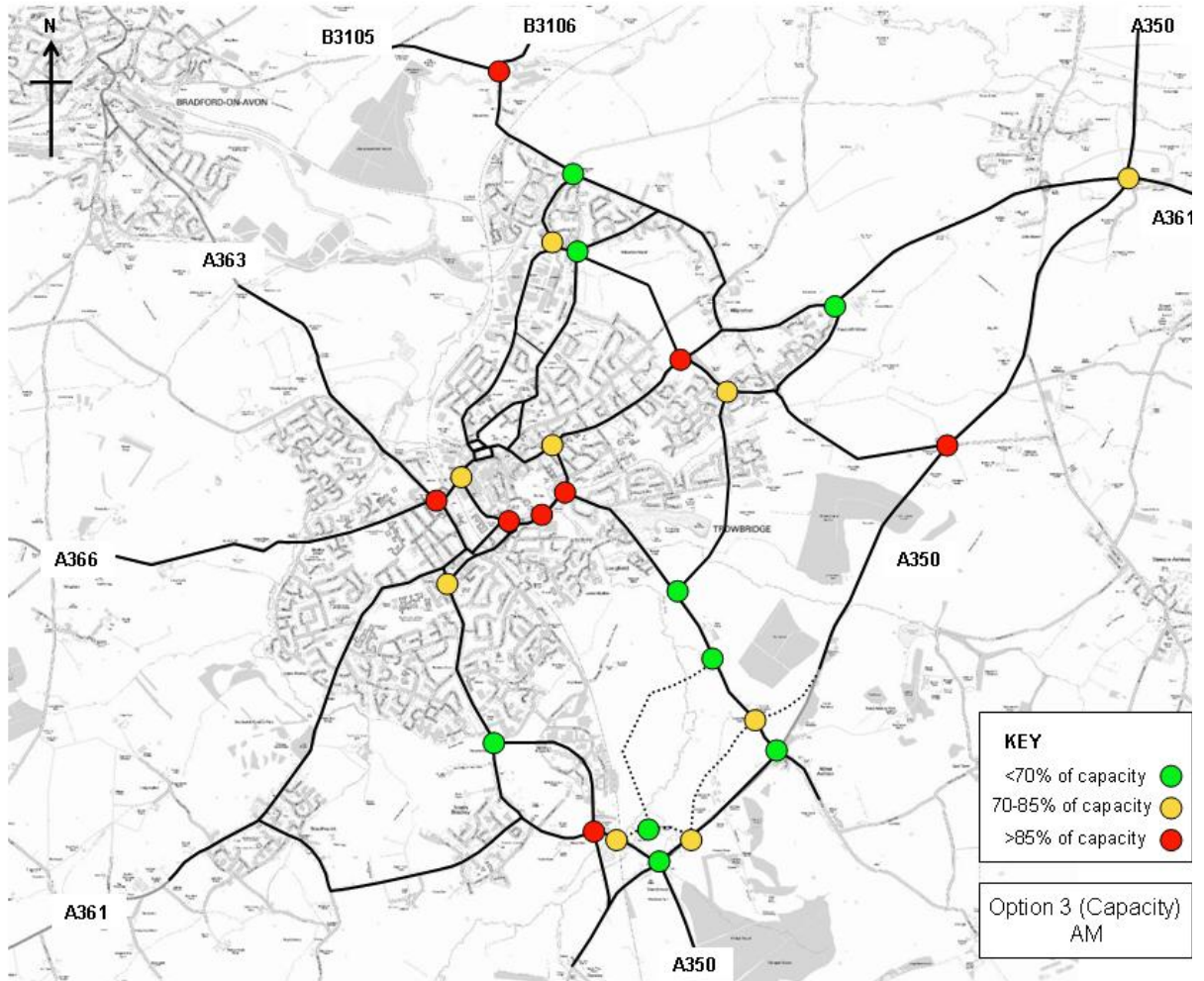
Figure D.9: Development Scenario 1: Option 3 Highway Capacity - Junction Capacity Summary AM Period
