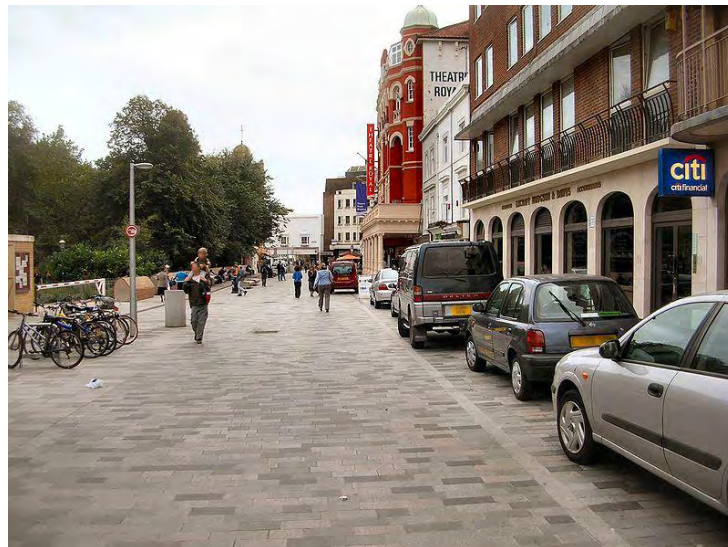
Figure 5.1 – Shared Surfaces (New Road, Brighton)
