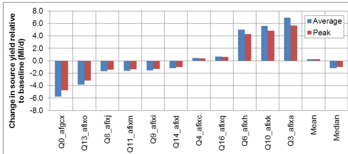
Figure 4-37: Summary of impact of climate change scenarios on average and peak yields hydrologically constrained groundwater sources
