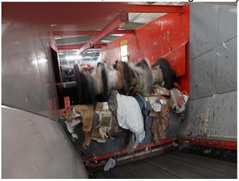
2. Shredded paper within MRF, not captured by the sorting process, and increasing dust and fire risk.
