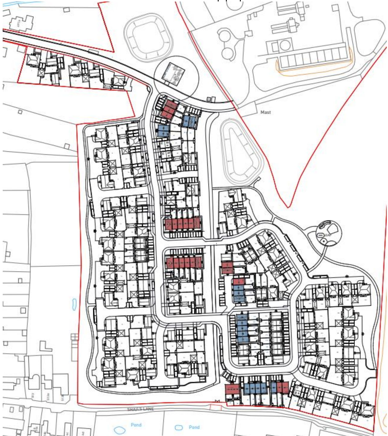
Affordable housing provision (Drg no. P21-3414_09 rev E) with red coding representing A/H rent and blue coding representing shared ownership properties.
